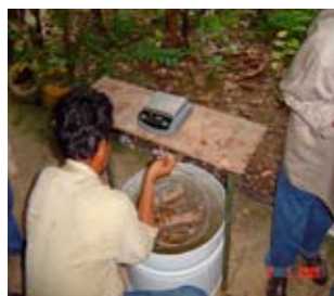
Weighing sample in air ( W_a ) and Weighing sample in water ( W_w ). Photos from CIAT
