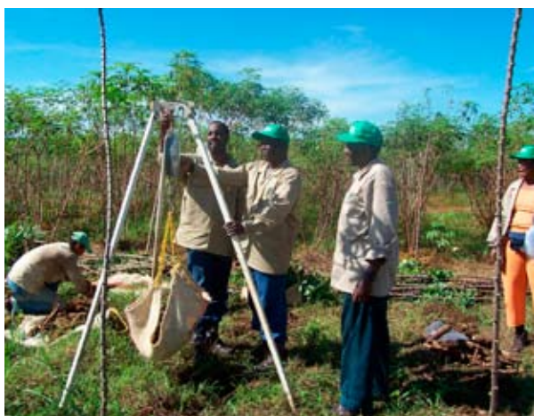
Weighing sample in air ( W_a ) and Weighing sample in water ( W_w ). Photos from CIAT
